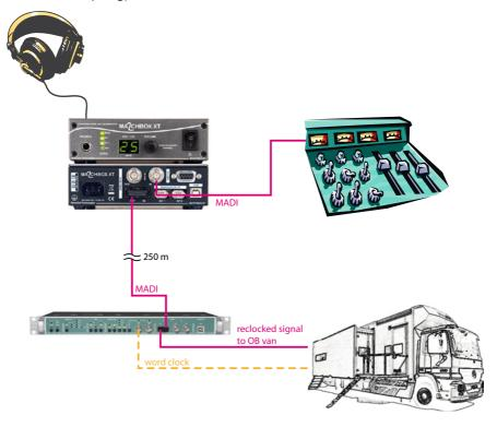
The (mostly) remaining fiber string could be used to return a control signal to the optical input. In case the coaxial input fails the box will switch to the other MADI input making a loop between OB van and stage then.
