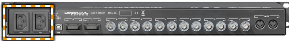
The left socket is switched by the power supply switch. The right socket will power up the device immediately when connected to the mains.
