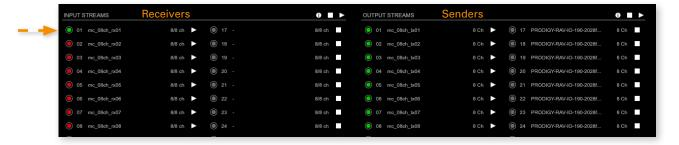
The status of an input stream changes (led green = stream active, receiving data) once this receiver has been patched to a sender.
