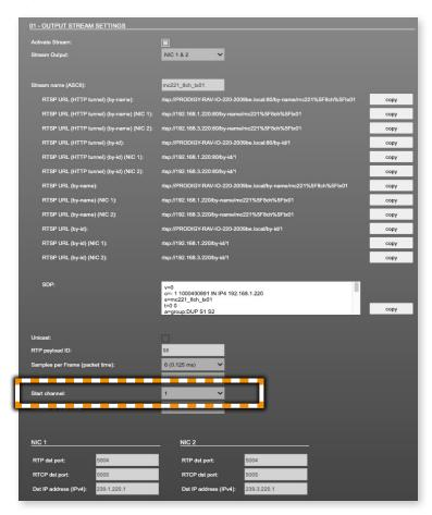
The 'start channel' is dynamically selected by HOME, depending on the number of audio channels occupied in the previous streams.
