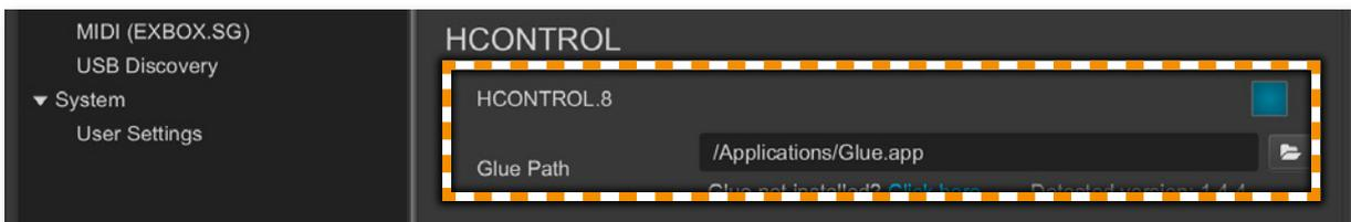
**5.** Check installation path of glue and activate HCONTROL (blue check box)
