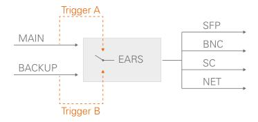
To override automatic switching temporarily the source can be forced to MAIN or BACKUP.
