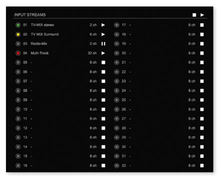
The module can subscribe up to 32 streams. The overview displays the basic information of each stream. The input stream name can be set manually (discovery protocol: manually, see p 58) overriding the SDP's stream name information.
