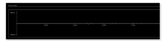
Graphical display of measured PTP jitter.
