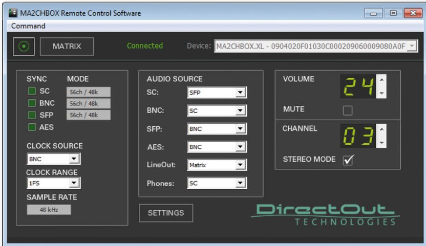
The overview informs about the input signal state and offers access to the clock setting, signal routing and the volume level and channel selection.
