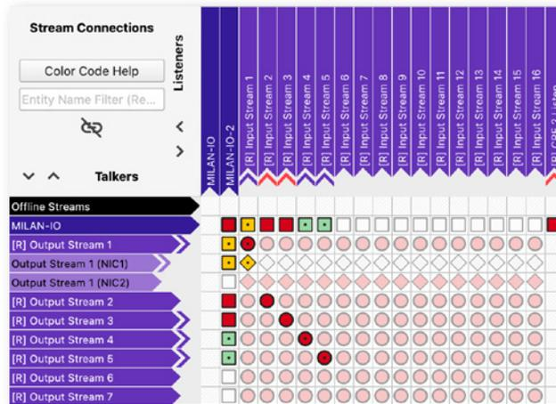
Output Stream 1 is expanded to modify single patches, patched to NIC 1 only. Output Stream 2 is patched to NIC 1 & 2.
