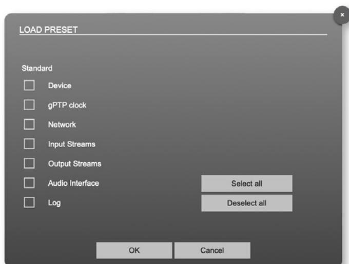
The device configuration can be stored to a single file (.rps). When restoring the configuration a dialog prompts for selection of individual settings. This enhances flexibility at setup changes when a particular adjustment shall be preserved or just a single adjustment shall be restored.
