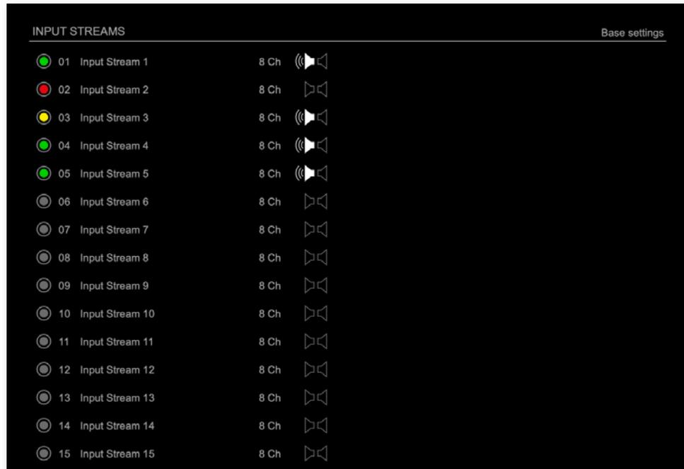
The module can subscribe up to 32 streams. 16 streams are enabled as factory default to avoid overlapping of I/O channels with 8 channel streams (128ch max). Each stream can be configured to contain between 1 and 8 audio channels. The overview displays the basic information of each stream. The input stream name must be set manually.
