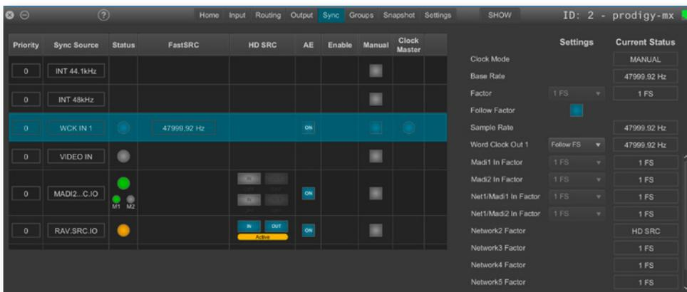
\*\*\* Word Clock input also accepts analog video signal (black burst, tri-level)
