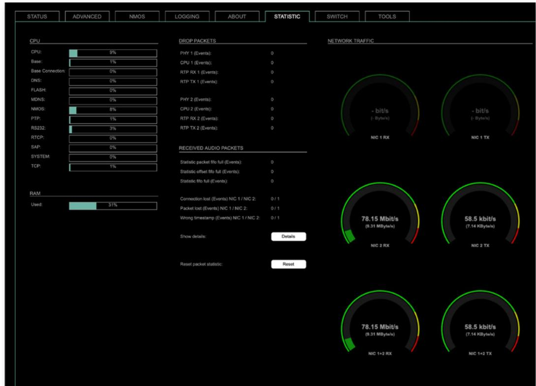
The tab 'STATISTIC' displays an overview of the CPU load of the particular processes, an error counter and a monitor display to indicate the incoming (RX) and outgoing (TX) network traffic on both network ports individually.
