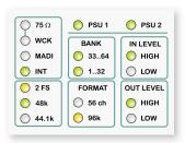
Clock source is set to internal clock generator. Conversion of channels 01-32 (i.e. all channels)\*.
