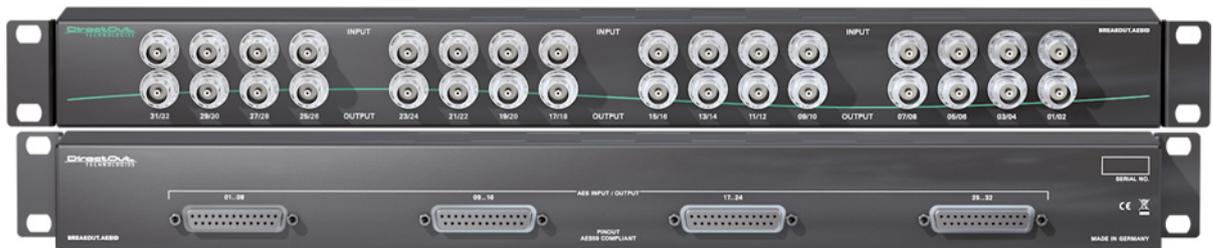
BREAKOUT.AESID- digital input / output, 16 AESid ports (32 channels)
