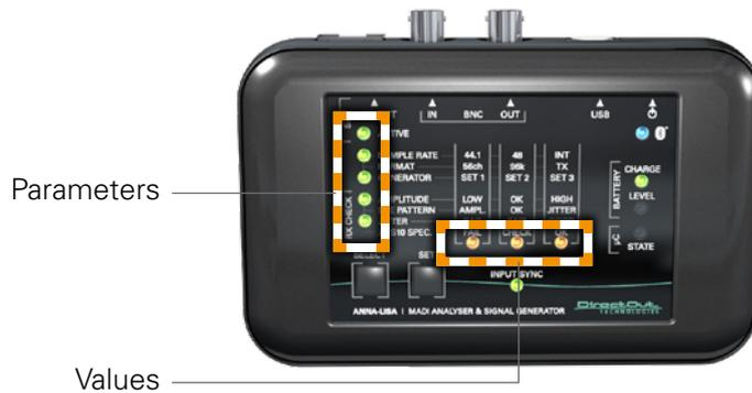
The LEDs in the column indicate the **parameters**.
