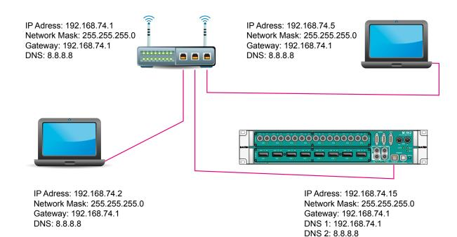
Three devices are connected by a router that handles the traffic within the network. Each device has its own <ip address>.
