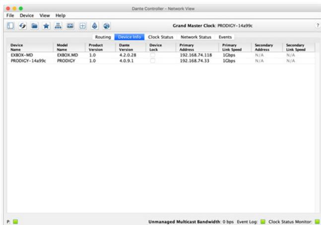
The DANTE.IO is delivered with the network interface set to DHCP as a default. Dante Controller can be used to discover the device on the network and change the IP configuration if necessary - see "Network Config" on page 8.
