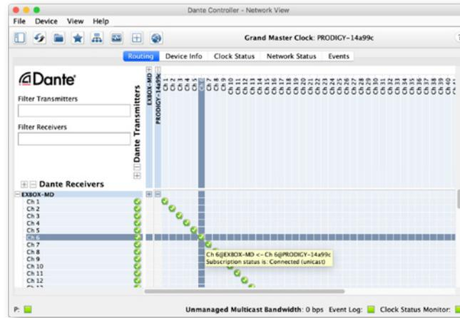
'Dante Receivers' in the vertical column displays the receiving devices (= destinations).
