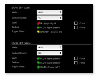
EARS is available for all four input ports (BNC, SC, SFP, NET) and with full routing support.
