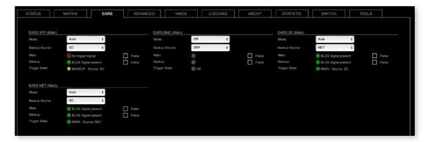
EARS™ (Enhanced Automatic Redundancy Switching) is a system to prevent interruption of the output signal. It uses either the proven BLDS™ technology or pilot tone triggering. A logic monitors the condition of the trigger signal on the input. In case of a failure it switches automatically to the backup input.
