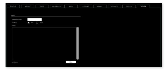
The tab 'TOOLS' offers a generator to ping any IP address (IPv4) from either NIC 1 or NIC 2. The result is displayed at the 'Output'.
