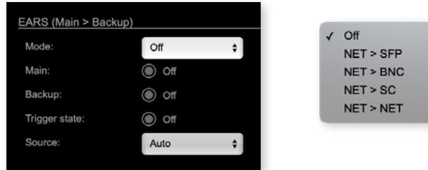
EARS™ (Enhanced Automatic Redundancy Switching) is a combination of DirectOut’s successful BLDS™ technology and pilot-tone based switching. A logic monitors a trigger signal contained in certain audio channels of the NET (RAVENNA) and MAD1 input.
