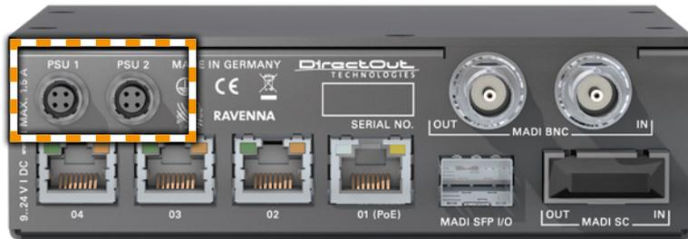
This device may operate with only one power supply. To provide power supply redundancy, it is recommended to connect both PSU 1 and PSU 2 to independent power supplies with separate fuses.
