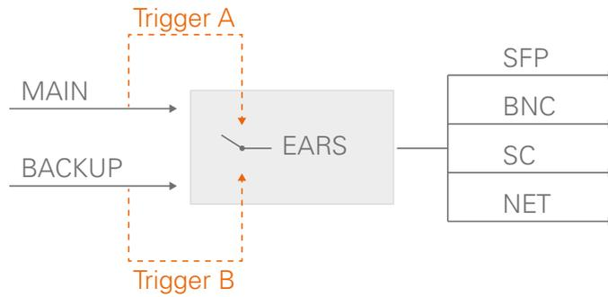
To override automatic switching temporarily the source can be forced to MAIN or BACKUP.
