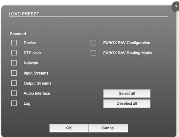
The device configuration can be stored to a single file (.rps). Restoring the configuration a dialog prompts for selection of individual settings. This enhances flexibility at setup changes when a particular adjustment shall be preserved or just a single adjustment shall be restored.
