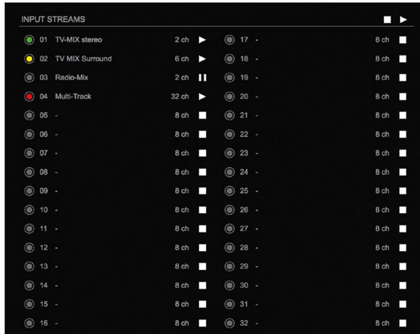
The module can subscribe up to 32 streams. The overview displays the basic information of each stream. The input stream name can be set manually (discovery protocol: manually, see p 58) overriding the SDP's stream name information.
