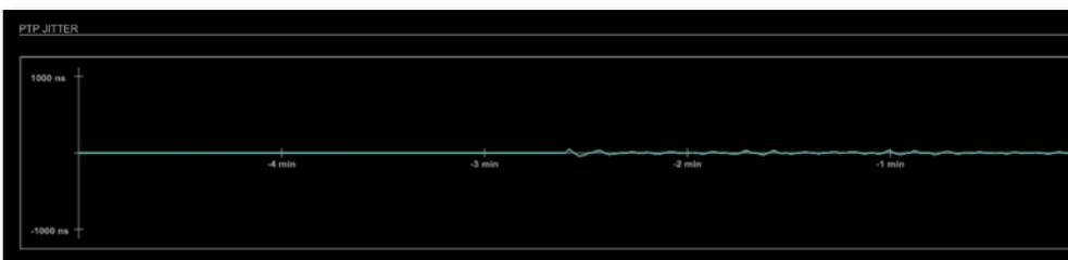
Graphical display of measured PTP jitter.
