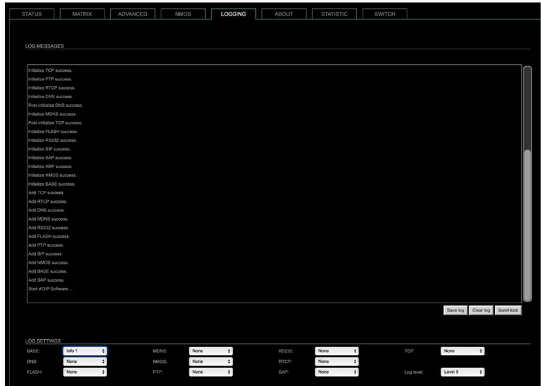
The tab 'LOGGING' displays logging depending on the 'Log Settings'. The logging can be enabled individually for different protocols, each of with an adjustable filter. An adjustable log level specifies the information detail of each entry.
