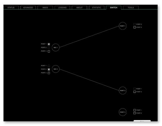
Two independent network interfaces (NICs) can be configured in the switch configuration.
