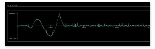
Graphical display of measured PTP jitter.
